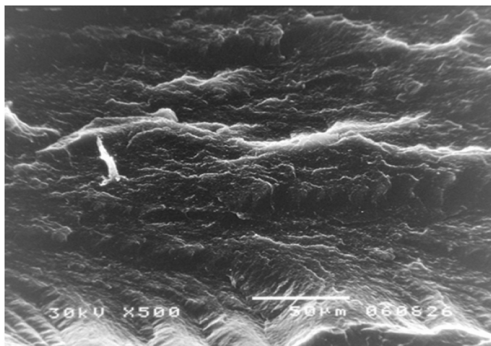
Figure 19. SEM micrograph of NBR/EPDM rubber blend filled with 70 phr carbon black (magnification X=500).
